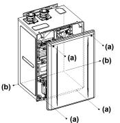
Assemble the 4 Brackets into the Side Covers referring to the following instruction.
